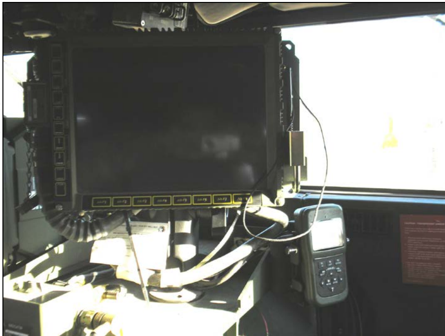
Figure 7-3. Blue Force Tracker Display Unit with the Defense Advanced GPS Receiver (DAGR)
